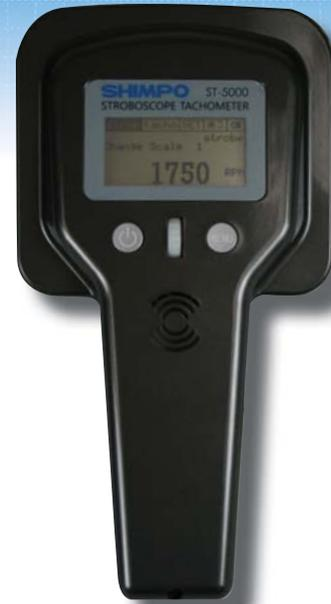
The ST-5000's LED technology extends operation due to the low energy requirement of the light diodes compared with xenon stroboscopes. Its large, backlit display and convenient 2 button plus dial wheel operation enable quick function selection. The scroll dial allows fast adjustment of flash rate and can adjust the rate multiplication factor (up to a factor of 10) to quickly scroll through the entire flash range.
